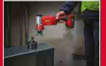
CONNECT - grab the tool and snap it on to the quick connect
