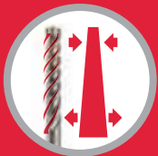
VARIABLE FLUTE GEOMETRY FOR FASTER DRILLING
